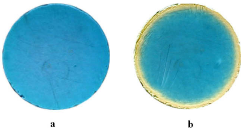
PLATE 1 a) Photographs of the thin film of pentacene at ambient pressure; b) photographs of the thin film of pentacene applying shear stress of less than 2 GPa.
